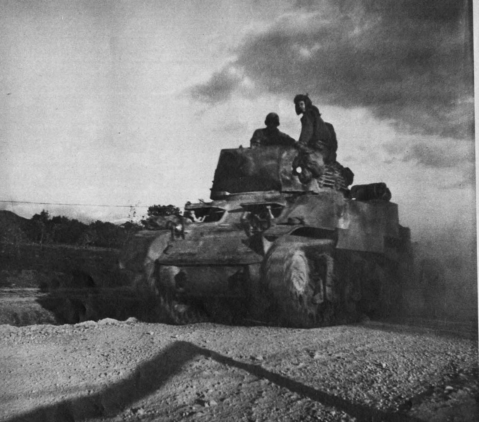
The M-8 self-propelled howitzer is one of the fastest full-track gun carriages in use, thanks to its M-5 light tank chassis. The similarity in appearance to the M-5 is very strong, breaking down only in the short,
